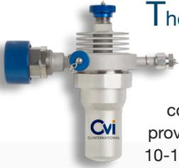
**The Finned Double-Cup Sampler** - This all stainless steel, machined and welded assembly contains a threaded double cup, a Burst Plug providing overpressure protection and a Charging Valve to trap the liquid sample once the system is cooled down. The finned design of this sampler provides improved vaporization (heat transfer) characteristics so as to enable 10-12 minute average sample time.
