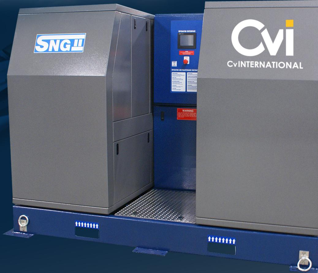
The SNG-II is a fully integrated, electronically driven, turn-key nitrogen generating system capable of producing nitrogen gas up to 99.9% purity at 8 to 25 scfm. Service pressures provided to 5000 psi with an option to 6000 psi.
