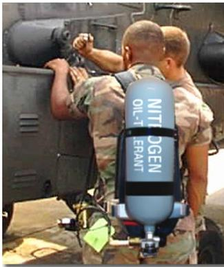
High Pressure Nitrogen Portable to “Point of Need” - 4500 psig Lightweight Backpack Cylinder - Part Number: 410780 and Harness - Part Number: 410735-1
